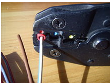
A wire and connector being crimped together with a crimping tool
