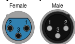
XLR connector , showing the notch for alignment
