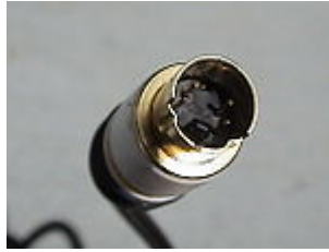
A 4-pin Mini-DIN S-Video cable, with notches and a rectangular alignment pin
