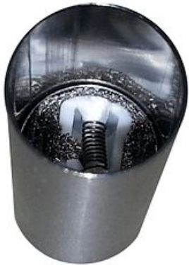
Inside view of an e-cigarette atomizer with the coil ( heating element ).
