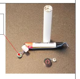
The **tubular electronic inhaler** includes an air-flow sensor which is a diaphragm microphone. Blowing across the sensor activates the power supply.
